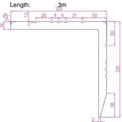
Wooden Composite L Profile 120 product is composed of at least 60% wood sawdust, 30% HDPE (high density polyethylene),
